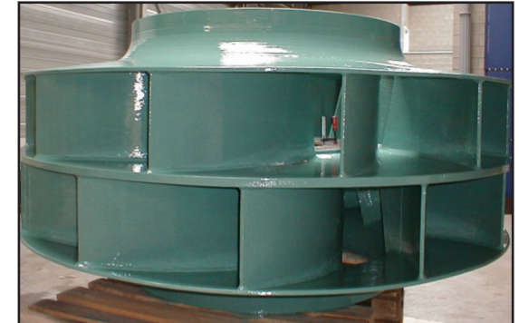
Two different fan impeller designs were upgraded with ARC S2 at 30 mils (750 µm)
